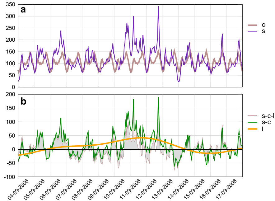
Fig. 1. Illustration of the filtering procedure for NO 2 hourly concentrations near Paris, along the “Boulevard Périphérique” (AirBase station FR04053). The first panel shows the row series (s) and the diurnal cycle (c) averaged over a sliding 31-day window centred on the considered day. The second panel shows the series filtered from the diurnal cycle (s-c), the signal filtered from the frequencies higher than 3 days (s-c-l), and the low frequency residual (l).
